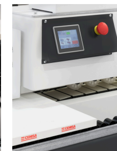
Control Panel Touchscreen 3,5" Industrial PLC
