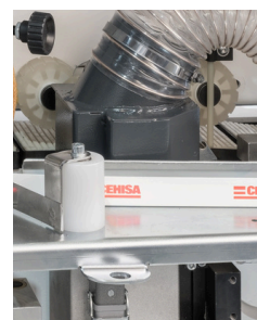
Pre-milling station w/ DIA tool
