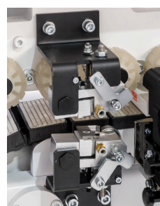
Glue Scraper station w/ floating blades
